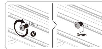
Note: Install seat supporter to the frame with the last two sliding nuts.
