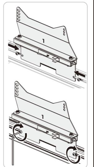
Insert **Pull Rod (J)** into the rails while keeping it aligned with the correct hole and clip.
