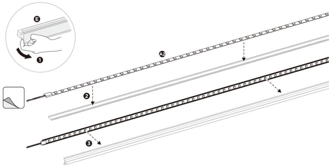
Remove the cover of side column, and assemble LED lighting strip into the column.
